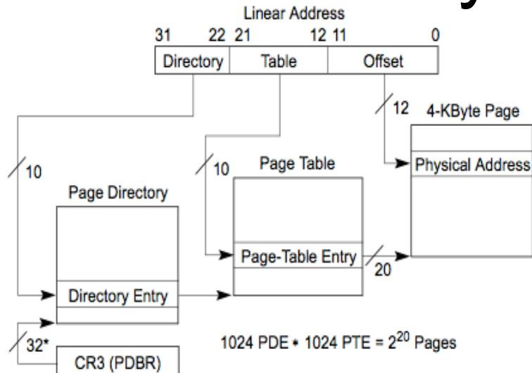
\*32 bits aligned onto a 4-KByte boundary.
