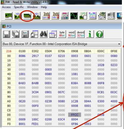
Therefore, with FWH\_DEC\_EN bit 14 asserted, we're decoding to a portion of BIOS binary  Click Memory button and type address FFF00000
