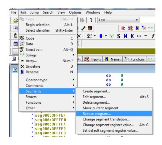
If you encounter a size-related error, open the binary file with a hex editor (like HxD) and delete the last byte. Then re-open the binary in IDA and rebase it. Still treat it like it were its original size.
