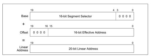
Figure 20-1. Real-Address Mode Address Translation
