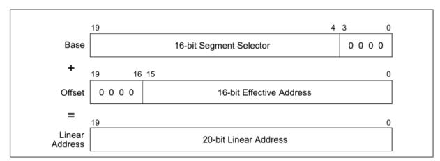
Figure 20-1. Real-Address Mode Address Translation
