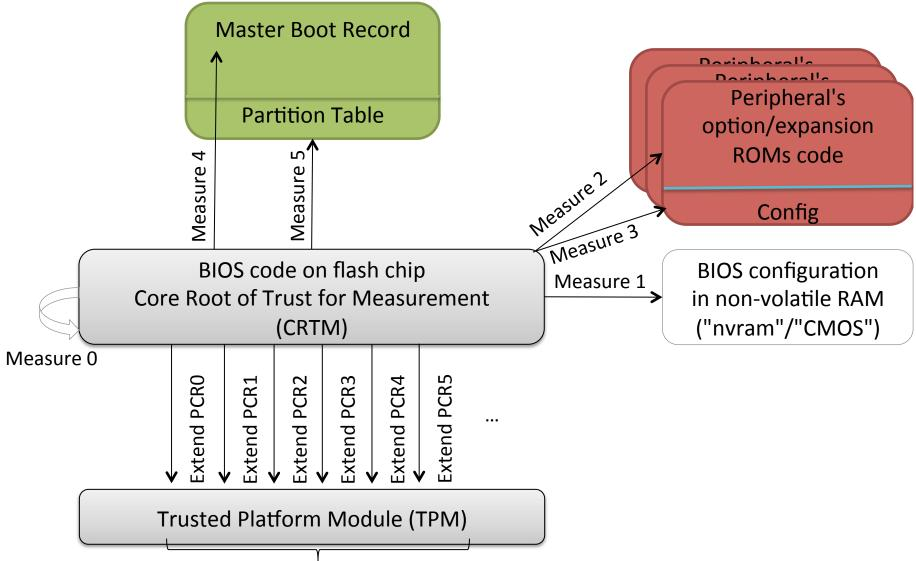
This collection of measurements going forward is the Static Root of Trust for Measurement (SRTM)
