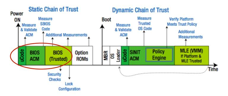
Figure 1-1. Intel<sup>®</sup> TXT launch timeline with static and dynamic chain of trust
