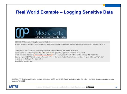
If an attacker can gain access to the system, then they can read this log and learn the password. Maybe MediaPortal isn't a critical system, but if a user is reusing their password on some other system then the attacker has just obtained credentials for that system.
